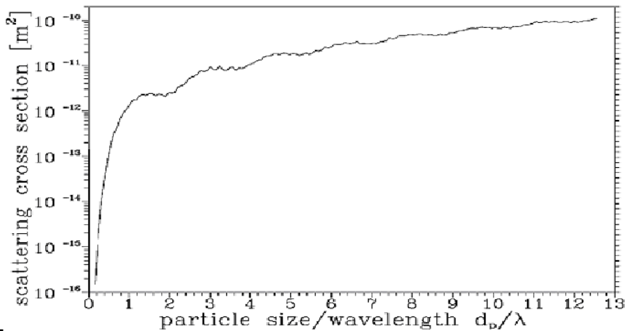
Figure 3.1: The scattering cross section as a function of particle size (refractive index m = 1.6 ) [3]
